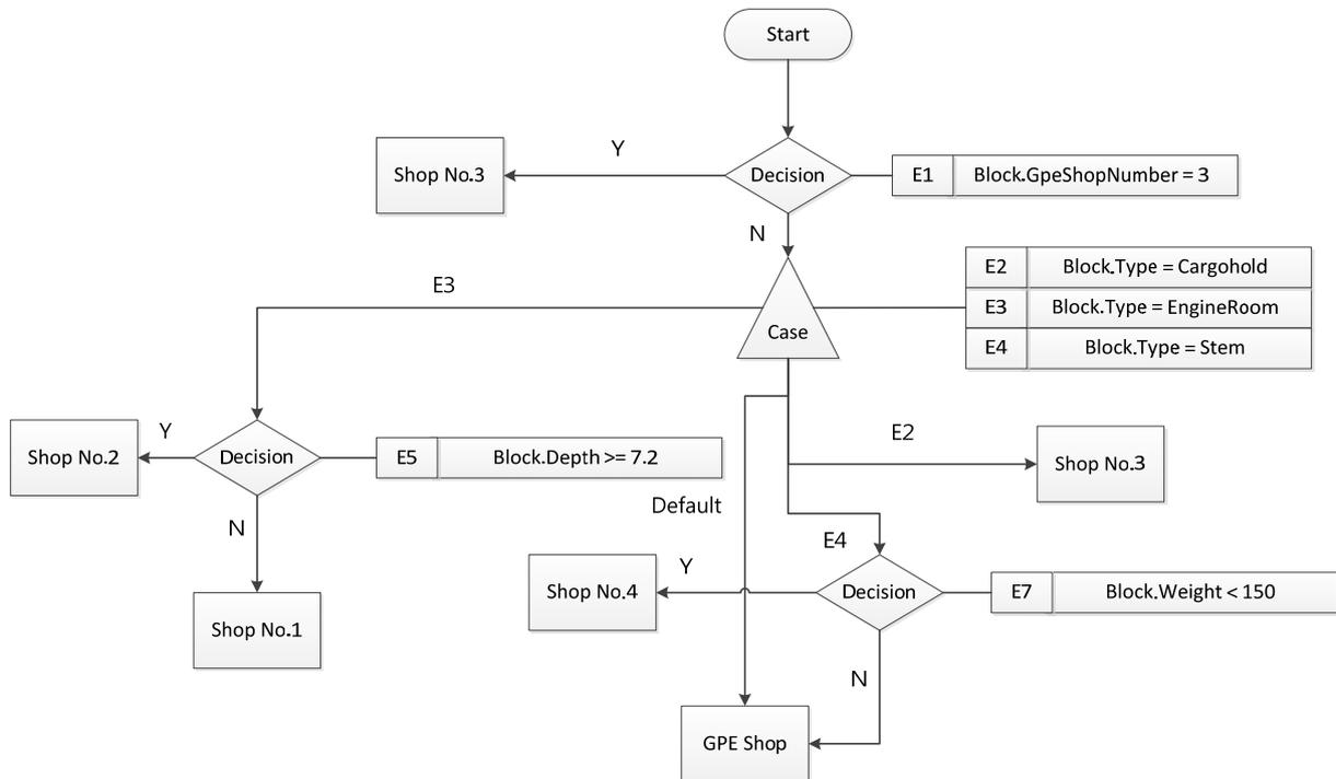
Fig. 7 Block assignment scenario model (1).
