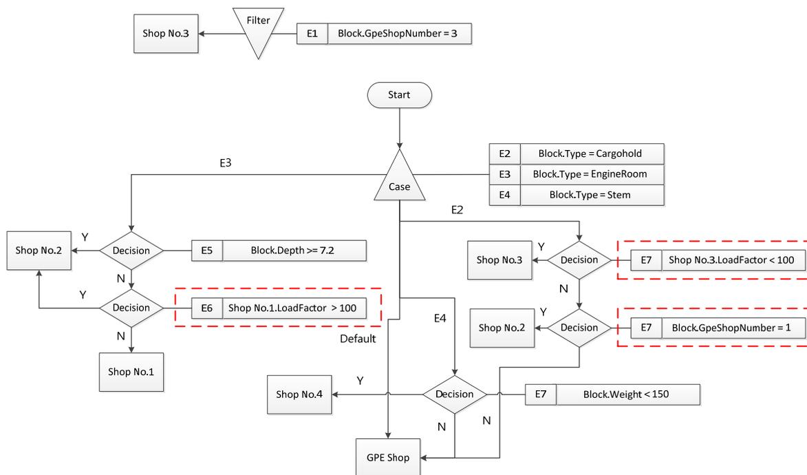
Fig. 8 Block assignment scenario model (2).
