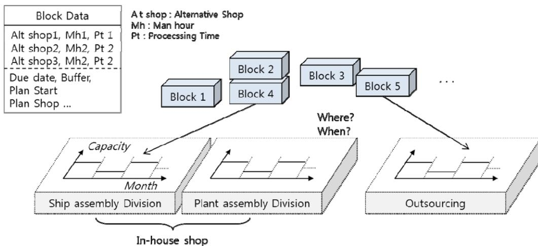
Fig. 1 Concept of block assignment planning.
