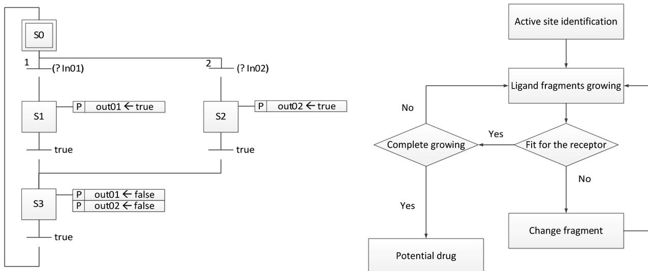
Fig. 3 Example of SFC (left) and flow chart (right).
