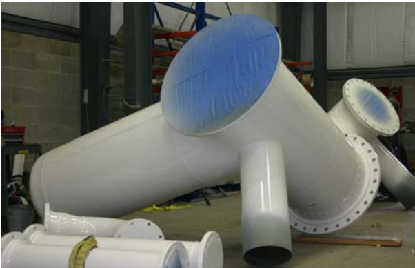
Fig. 1 Pipe spools used at offshore plant
