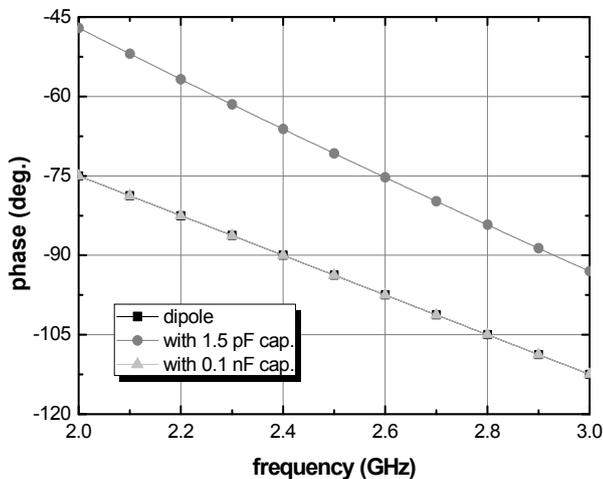
Fig. 4. Electrical lengths of the parasitic elements with and without reactive components.
