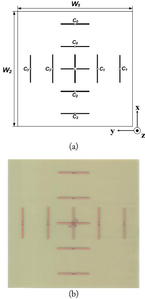
Fig. 5. Proposed four-way planar Yagi-Uda antenna. (a) Layout of the proposed antenna. (b) Photograph of the fabricated antenna.
