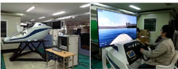
Fig. 4 Sample of a leisure boat simulator
