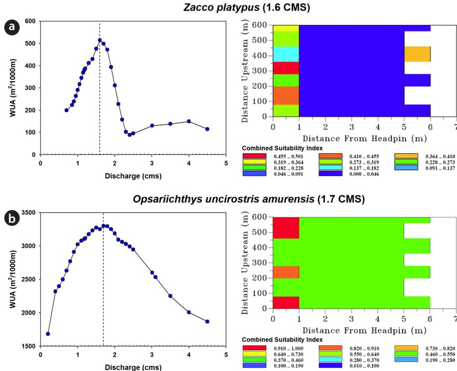
**Fig. 3.** Plotted by PHABSIM, weighted usable area (WUA) (left) varying with changes in discharge of (a) *Zacco platypus* and (b) *Opsariichthys uncirostris amurensis*. Dotted lines indicate flow rates that showed the widest WUA. Combined suitability index (CSI) of fishway cells applied to the highest WUA of the two species. A headpin is a control point when measuring fishway widths of a certain section, and we measured widths from the left sides of fishway.
