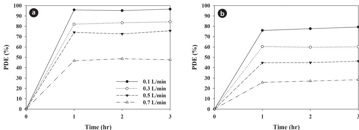
**Fig. 7.** Photocatalytic degradation efficiencies for (a) trichloroethylene and (b) perchloroethylene as determined using a LED-activated N-TiO<sub>2</sub> photocatalytic system according to stream flow rate (0.1, 0.3, 0.5, and 0.7 L/min). LED: light-emitting diode, N-TiO<sub>2</sub>: N-doped titanium dioxide, PDE: photocatalytic degradation efficiency.
