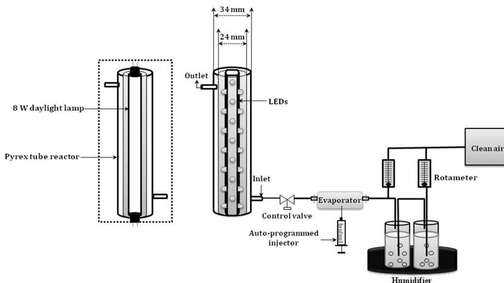
Fig. 1. Schematic diagram of experimental set-up. LED: light-emitting diode.
