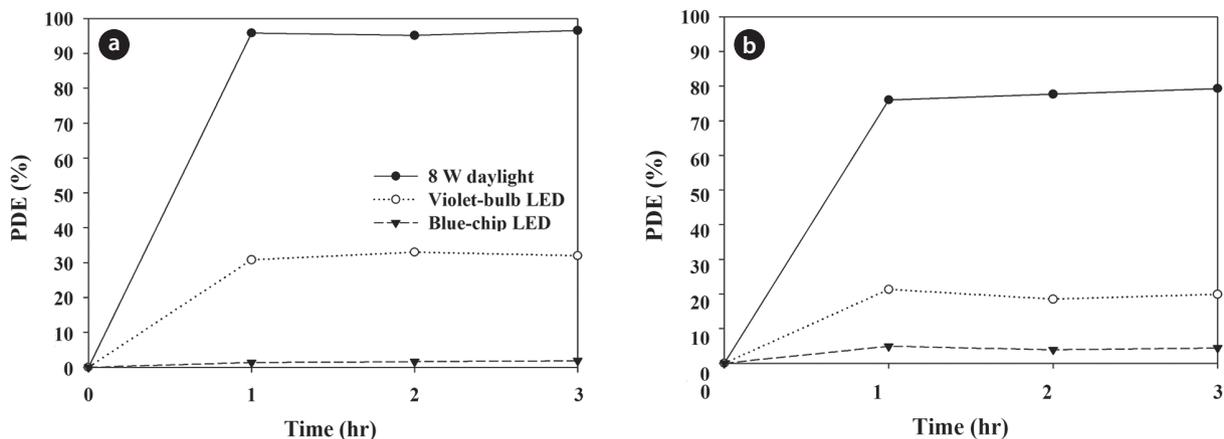
**Fig. 5.** Photocatalytic degradation efficiencies for (a) trichloroethylene and (b) perchloroethylene as determined using a LED-activated N-TiO<sub>2</sub> photocatalytic system according to lamp type (8-W fluorescent daylight lamp, blue- and violet-LEDs). LED: light-emitting diode, N-TiO<sub>2</sub>: N-doped titanium dioxide, PDE: photocatalytic degradation efficiency.
