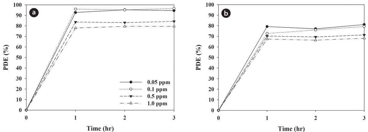
**Fig. 6.** Photocatalytic degradation efficiencies for (a) trichloroethylene and (b) perchloroethylene as determined using a LED-activated N-TiO<sub>2</sub> photocatalytic system according to input concentrations (0.05, 0.1, 0.5, and 1.0 ppm). LED: light-emitting diode, N-TiO<sub>2</sub>: N-doped titanium dioxide, PDE: photocatalytic degradation efficiency.
