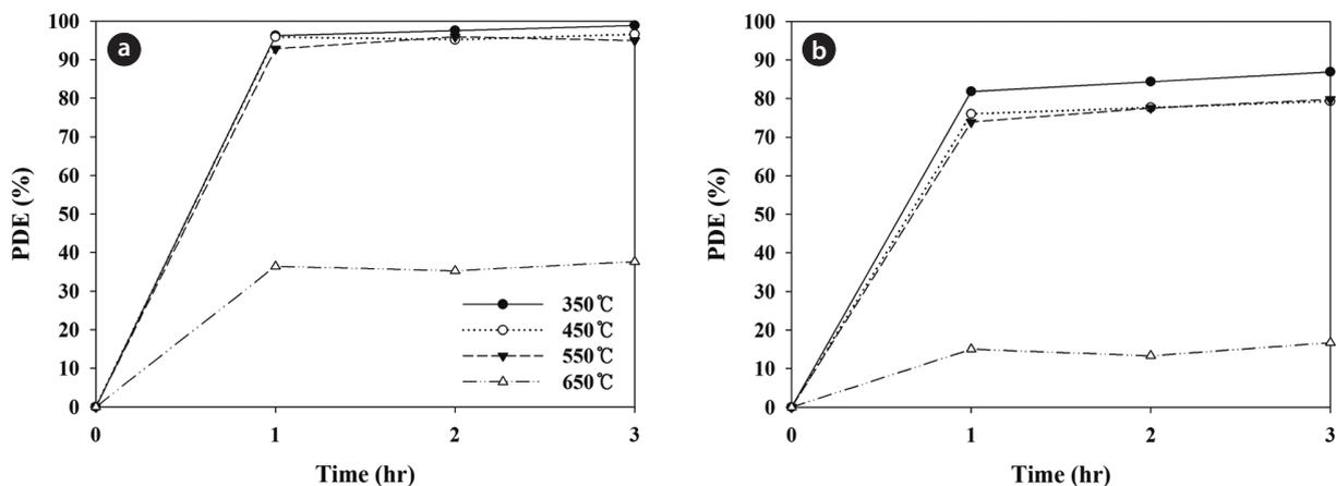
**Fig. 2.** Photocatalytic degradation efficiency of (a) trichloroethylene and (b) perchloroethylene, as determined via a photocatalytic system with N-TiO<sub>2</sub>, according to calcinations temperature (350°C, 450°C, 550°C, and 650°C). N-TiO<sub>2</sub>: N-doped titanium dioxide, PDE: photocatalytic degradation efficiency.
