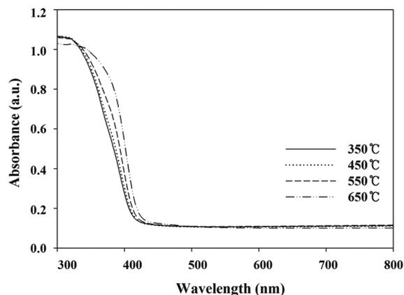
**Fig. 3.** UV-visible spectra of N-TiO<sub>2</sub> photocatalysts calcined at four different temperatures (350°C, 450°C, 550°C, and 650°C). N-TiO<sub>2</sub>: N-doped titanium dioxide.
