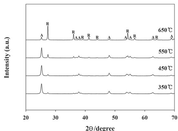
**Fig. 4.** X-ray diffraction patterns of N-TiO<sub>2</sub> photocatalysts calcined at four different temperatures (350°C, 450°C, 550°C, and 650°C). N-TiO<sub>2</sub>: N-doped titanium dioxide. A: anatase, R: rutile.
