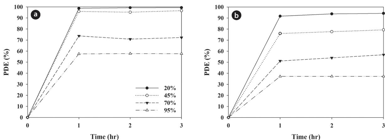
**Fig. 8.** Photocatalytic degradation efficiencies for (a) trichloroethylene and (b) perchloroethylene as determined using a LED-activated N-TiO<sub>2</sub> photocatalytic system according to relative humidity (20%, 45%, 70%, and 95%). LED: light-emitting diode, N-TiO<sub>2</sub>: N-doped titanium dioxide, PDE: photocatalytic degradation efficiency.
