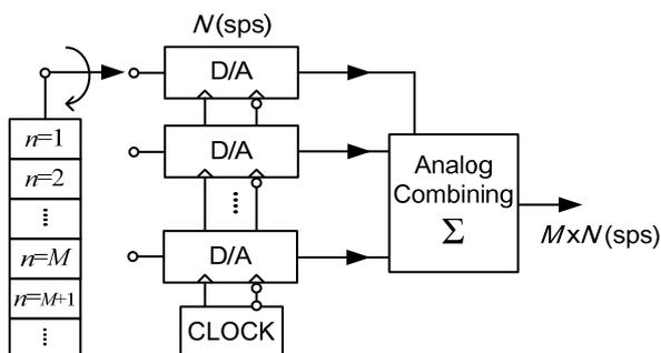
Fig. 1. Time-interleaving digital-to-analog converting system.
