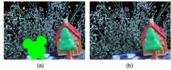
Fig. 4. Image restoration in synthetic aperture integral imaging. (a) The mask marked in green. (b) The occlusion removed from the elemental image.
