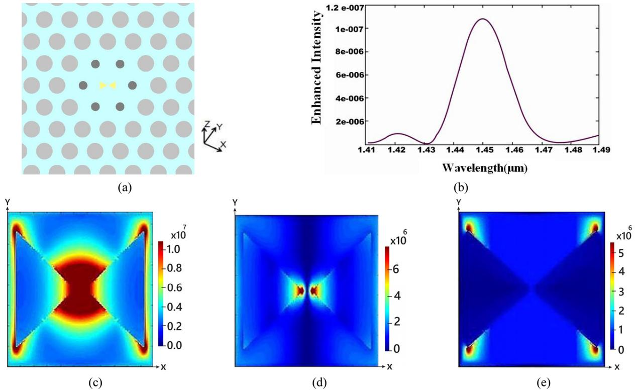
FIG. 4. (a) Two-dimensional view of the analyzed hybrid structure, (b) wavelength spectrum of the hybrid structure, (c) calculated enhancement of the electric field intensity distribution  $|E|^2$  at the resonant wavelength, (d) calculated enhancement of the  $x$ -component of the electric-field intensity distribution  $|E_x|^2$  at the resonant wavelength, (e) calculated  $y$ -component of the electric-field intensity distribution  $|E_y|^2$  at the resonant wavelength.
