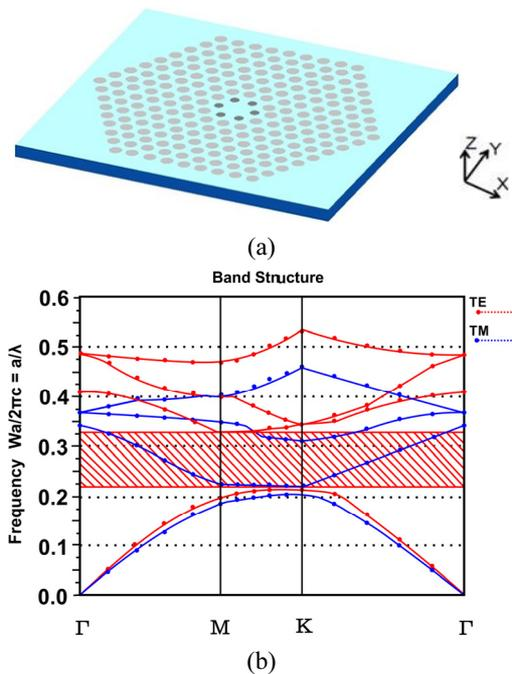
FIG. 1. (a) Three-dimensional view of the PC cavity (core area of PC nanocavity in dark gray, cladding in light gray), (b) band structure of the PC structure.
