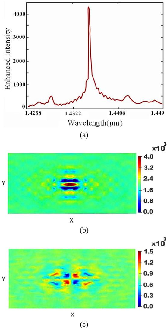
FIG. 2. (a) The spectrum of the PC nanocavity, (b) corresponding x-component of the electric-field intensity at the resonant wavelength, (c) corresponding y-component of the electric-field intensity at the resonant wavelength.
