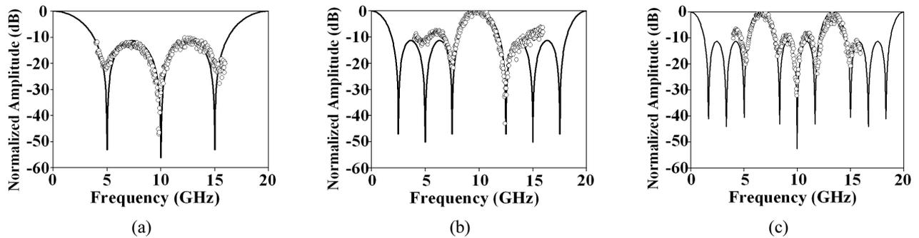
FIG. 5. The frequency responses of the proposed filter when  $V_{EOM1} = 2.0$  V,  $V_{EOM2} = 2.0$  V and the columns of the fiber optic delay line are in the (a) CROSS-BAR states (b) BAR-CROSS states (c) CROSS-CROSS states. Theory (solid line) and Experiment (hole).
