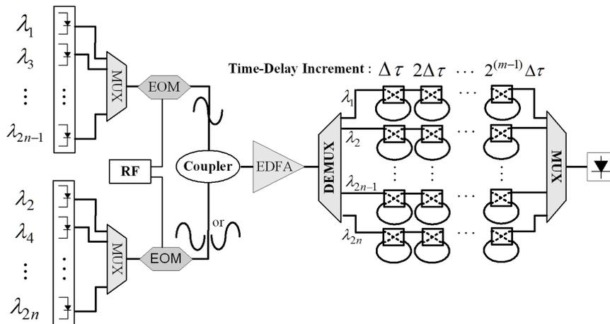
FIG. 1. Schematic diagram of the proposed fiber optic delay line based microwave photonic filter with negative or positive coefficients.
