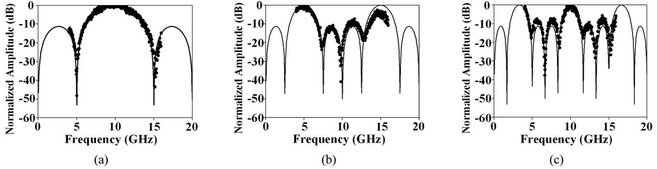
FIG. 4. The frequency responses of the proposed filter when  $V_{EOM1} = 2.0$  V,  $V_{EOM2} = 4.0$  V and the columns of the fiber optic delay line are in the (a) CROSS-BAR states (b) BAR-CROSS states (c) CROSS-CROSS states. Theory (solid line) and Experiment (dot).
