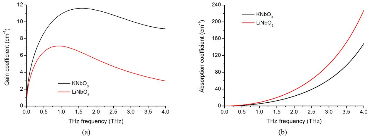
FIG. 7. THz-wave parametric gain coefficient  $g_T$  and absorption coefficient  $\alpha_T$  for KNbO<sub>3</sub> and MgO:LiNbO<sub>3</sub> at room temperature ( $\lambda_p = 633$  nm,  $I_p = 100$  MW/cm<sup>2</sup>): (a) gain coefficient  $g_T$ , (b) absorption coefficient  $\alpha_T$ .
