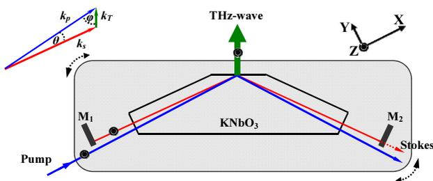
FIG. 1. Schematic diagram of a surface-emitting TPO using KNbO<sub>3</sub> with a noncollinear phase-matching scheme.
