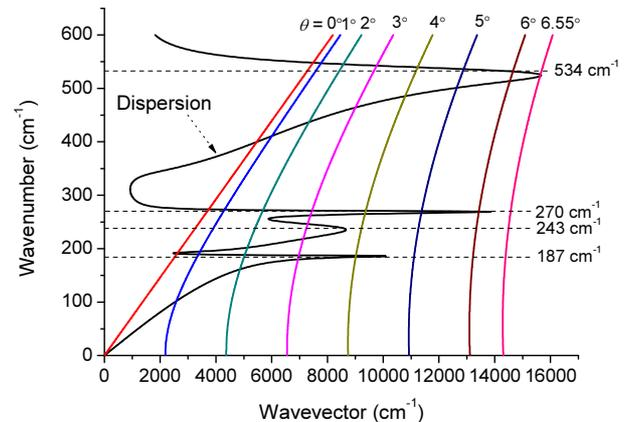
FIG. 2. Dispersion curve for the B<sub>1</sub>-symmetry polariton modes in KNbO<sub>3</sub> and the phase-matching curves for the 1064-nm pump laser.
