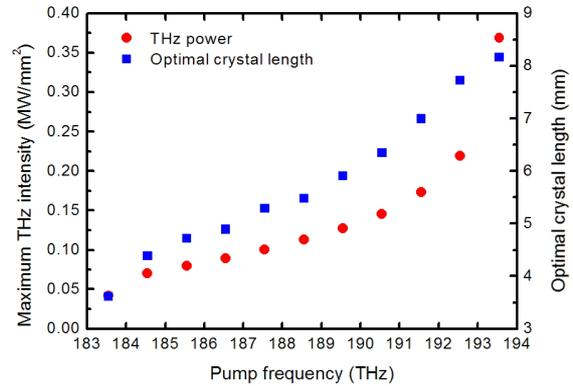
FIG. 5. The relationship between the maximum THz intensities and pump frequencies. Both the pump and signal intensities are  $20 \text{ MW/mm}^2$ .
