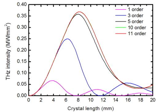
FIG. 3. THz intensities by GaP ridge waveguide based on cascaded DFG with cascading orders 1, 3, 5, 10 and 11.
