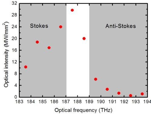
FIG. 4. The maximum intensity of the optical waves during the cascaded Stokes processes and anti-Stokes processes. Assuming the initial pump and signal waves are 188.55 and 187.55 THz with a power density of  $20 \text{ MW/mm}^2$ , respectively.
