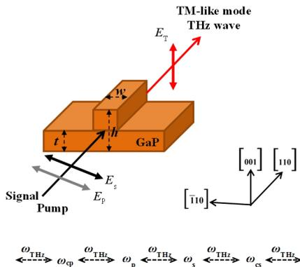
FIG. 1. Schematic diagram of the cascaded DFG to generate THz radiation by GaP ridge waveguide. DFG with Type-I phase matching condition, the electric field vectors of pump and signal wave  $E_p$  and  $E_s$  are along  $[\bar{1}10]$ , and that of THz wave  $E_T$  is along  $[001]$ .
