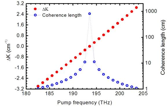
FIG. 2. Wave vector mismatch and coherence length of cascaded DFG. Assuming  $\omega_p = 193.55 \text{ THz}$ ,  $\omega_s = 192.55 \text{ THz}$ ,  $\omega_T = 1 \text{ THz}$ .
