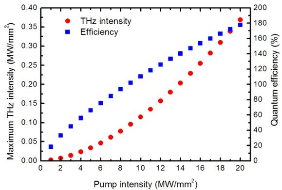
FIG. 6. The maximum THz intensity and quantum conversion efficiency versus pump intensity. Assuming pump and signal frequencies are 193.55 and 192.55 THz, respectively.
