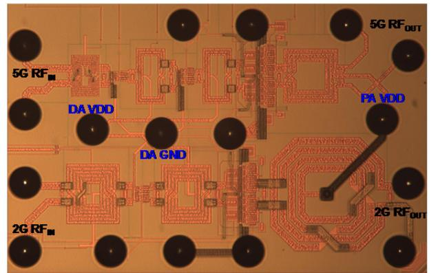
Fig. 7. Die photograph of the fabricated dual-band PA.
