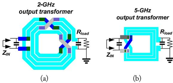
Fig. 3. (a) 2 GHz PA output transformer with input and output capacitors, (b) 5 GHz PA output transformer with input and output capacitors.
